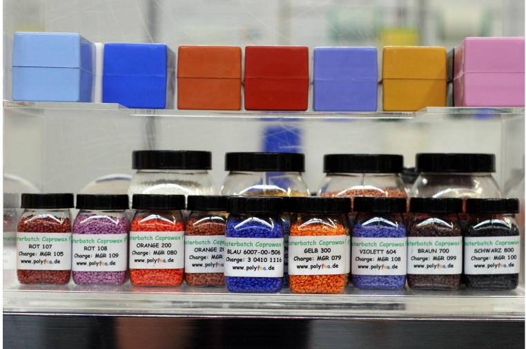
CAPROWAX P-Masterbatches for Bioplastics/ Biocomposites/Blends/Filaments: PLA, PBS, PHA, PCL, CAPROWAX  $P^{TM}$ /Blends, BioMineralComposites, Bio-NFC, Bio-WPC, Polysaccharides/Derivates, Casein, PVAc/Bioplastic-Blends, PVOH, Bio-TPE, Bio-UPR, NIPU. Carrier material based on CAPROWAX  $P^{TM}$  6006 is compostable, waterproof and according to DIN EN 13432. Customers request will be coordinated with toll manufacturer.
